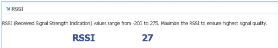
Figure 3 15. Antenna Pointing Pane
