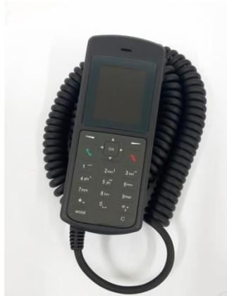
The Atlas IP Handset's connector is plugged into the BDU's handset port. It is powered directly from the BDU.
