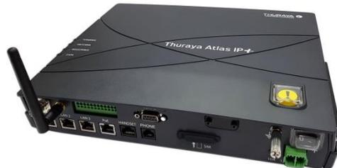
The BDU requires +12V or +24V DC power supply input. The BDU supplies the ADU via the single RF / coaxial antenna cable.
