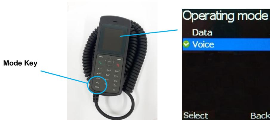
On handset's “**Mode**” key, press it to display the state of operating mode of “**Data**” or “**Voice**” on the handset display. Use Up/Down keypad to select the desired mode and then “**Select**” to activate it.
