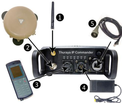
Figure 3: Hook-up Diagram (numbering same as above)
